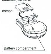
Remove the battery compartment cover and insert four
